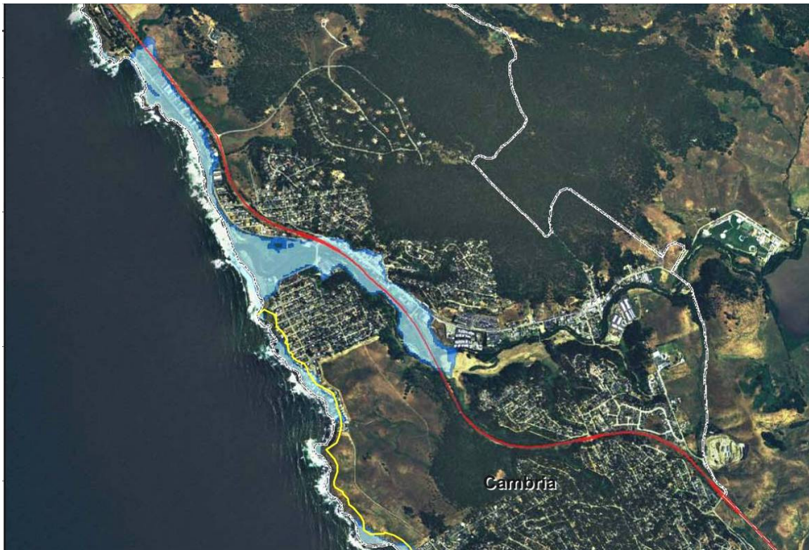
Figure 2-6. Predicted flood risk in 2100 in the Cambria area under a 1.4-m sea-level rise scenario. Light blue area is the current coastal base flood (approximate 100-year flood extent), dark blue area is the predicted coastal base flood under sea-level rise (current plus 1.4 m), yellow line is the predicted landward limit of erosion high hazard zone in 2100, and red line is Highway 1. Map used with permission from the Pacific Institute, Oakland, California.
