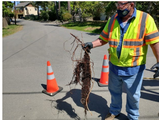
Figure C- Operator Delon Blackburn with a root ball retrieved from a wastewater collection system line.
