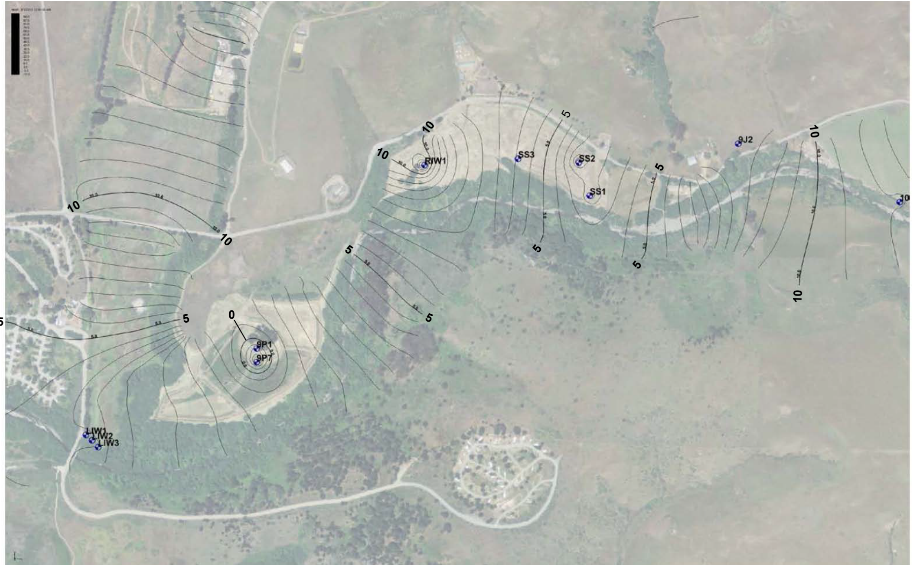
Figure 2 Simulated Groundwater Elevations After One Year of Operation
