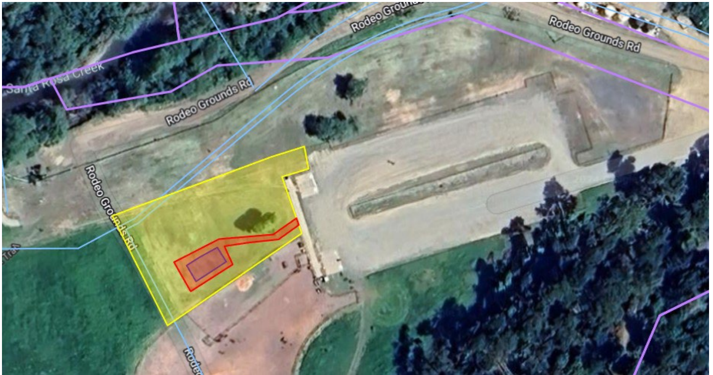
Figure 1 - Existing Site Overview. The whole construction area is in yellow, the sidewalk location is in red, and the restroom building location is in blue
